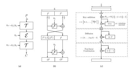
Figure 1: Proposed encasing for a block cipher  $\mathcal{E}$ , with key  $K_{\mathcal{E}}$  and block size *b*, within two keyed transformations  $\mathcal{T}$ , with key  $K_{\mathcal{T}}$ ,  $|K_{\mathcal{T}}| \ge |K_{\mathcal{E}}| \ge b$  (a), detail of the keyed transformation  $\mathcal{T}$  (b), and detail of the Feistel  $\mathcal{F}$  function in  $\mathcal{T}$ , taking  $I^l$ ,  $K_1$  as input (c)
