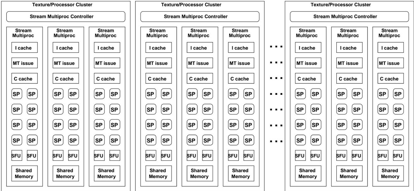
**Figure 1. Sketch of the NVIDIA GT200 streaming processors array architecture: each Texture/Processor Cluster contains three stream multiprocessors. In turn, each stream multiprocessor is composed of eight streaming processor cores (SP), plus two special function units (SFU). Shared memory is local to each stream multiprocessor.**
